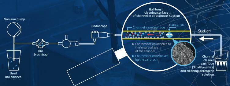
Micro balls, made of more than one million fibers with a size of a few microns, for an effective, safe, stable and fast channel brushing.
